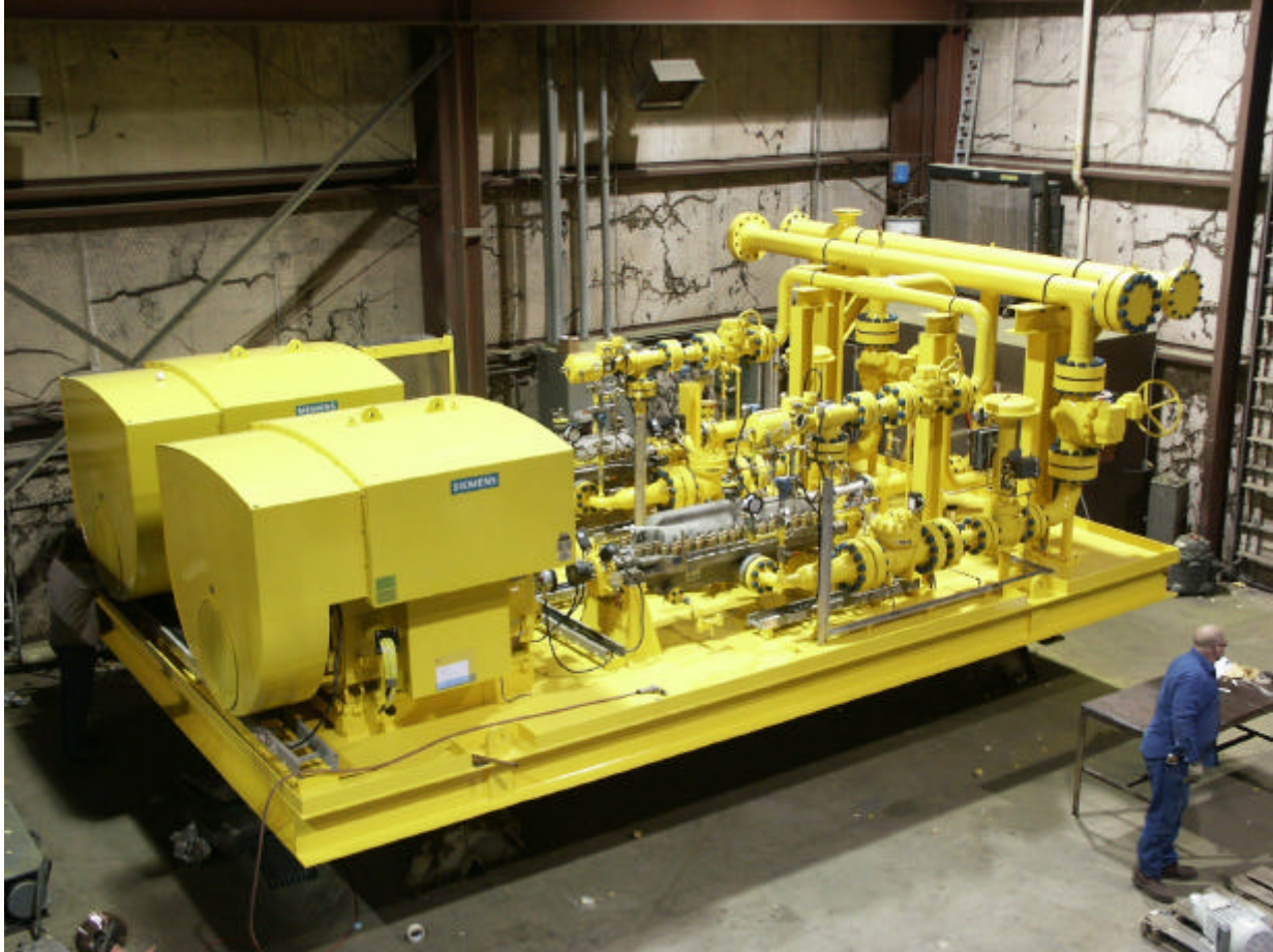
Seawater Injection Pump Module installed on FPSO in Offshore USA
