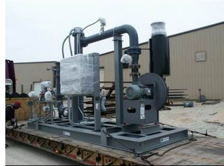
Ammonia Flow Control Package Customer: Sunoco Refinery
