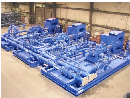
Water Injection Pump Package Customer: Chevron
