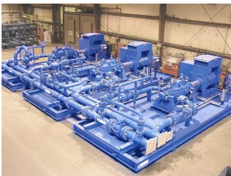
Water Injection Pump Package Customer: Chevron
