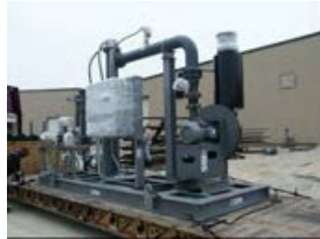
Ammonia Flow Control Package Customer: Sunoco Refinery
