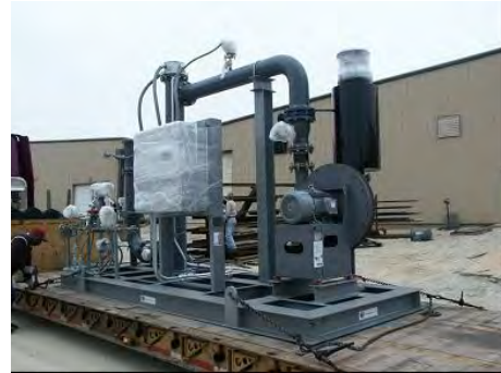
Ammonia Flow Control Package Customer: Sunoco Refinery
