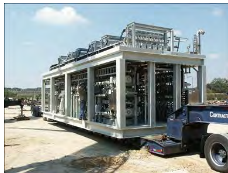
Chemical Injection Packages Customer: Chevron
