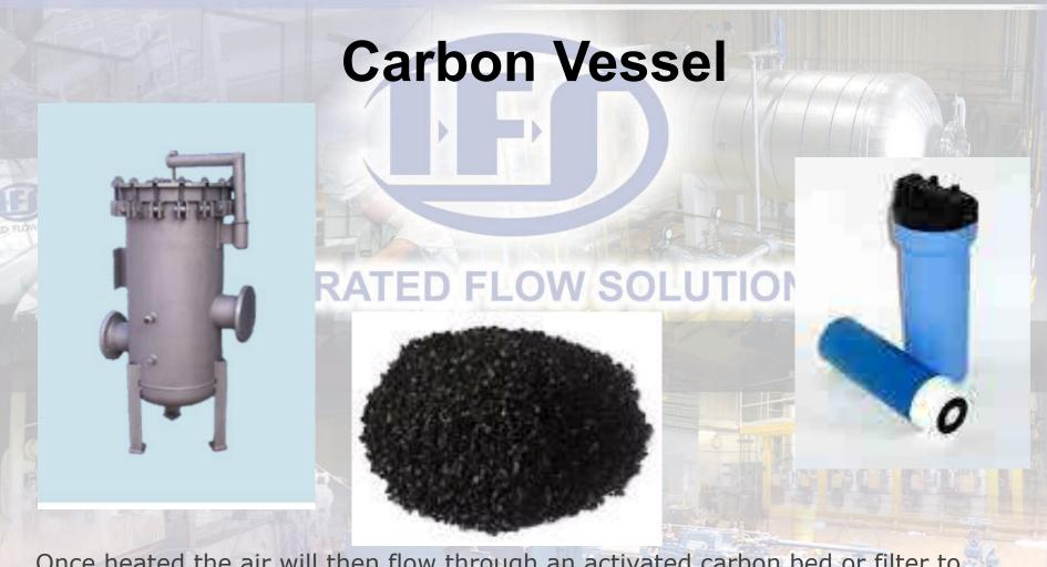
Once heated the air will then flow through an activated carbon bed or filter to remove any additional Hydrocarbon Vapors prior to entering the membranes.
