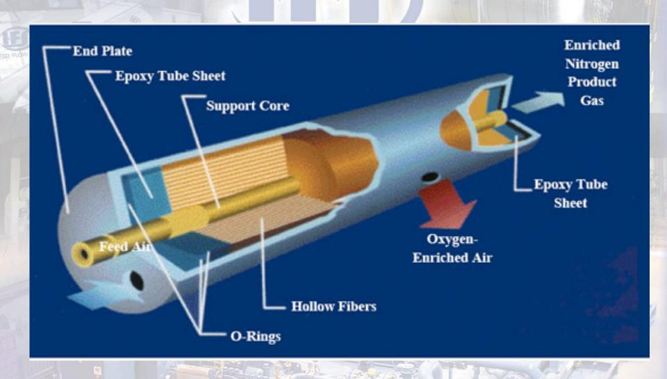
At the heart of the technology are polymeric membrane materials that allow for the rapid passage of one gas while minimizing the passage of another when applying pressure gradient across the membrane. This figure demonstrates the relative rate of common gases with the focus on the separation of O2 from compressed air to provide a high purity N2 stream. Membrane materials are formed into hollow fibers to provide high surface area for high volumetric gas processing rates.
