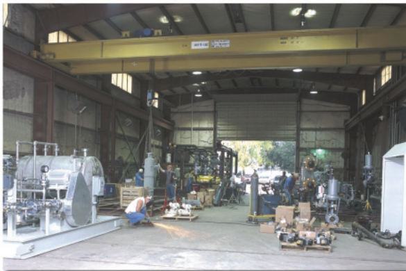
One of Seven IFS Fabrication Bays. Industry standards include vessels to ASME Section VIII, piping designed to ANSI B31.1/31.3 & fabricated to ASME Section IX, structural steel to AWS D1.1.
