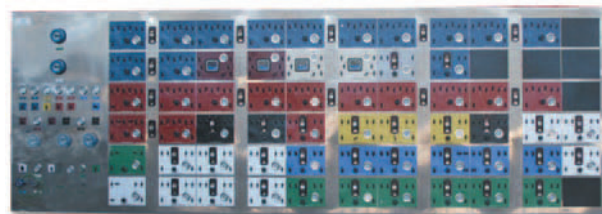
Injection Rate Control Panel
